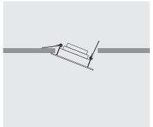
2. Secure the fixture frame by pushing in the other side.
