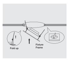
1. Cutout and fold up the spring clips and gently insert one side of the fixture frame into the cut out hole.
